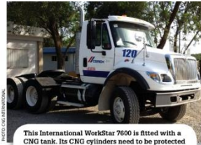
This International WorkStar 7600 is fitted with a CNG tank. Its CNG cylinders need to be protected from impact damage, road debris, and UV exposure from sunlight.
