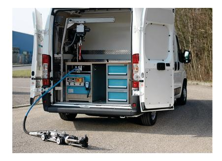
It's a CCTV van and the engine idles to provide power to the camera and other equipment needed for pipeline inspection. Plus, it's in a hot environment and the air-conditioned cab provides shelter for the technician.
