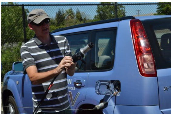
Refueling a fuel cell car with hydrogen
