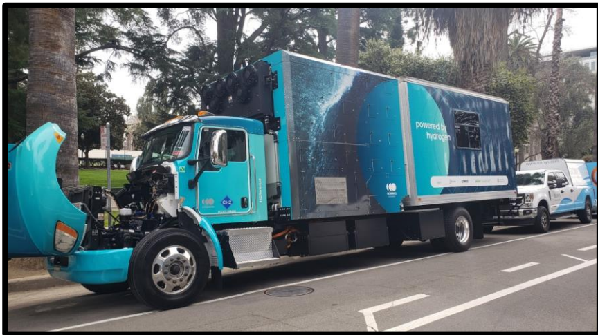
Cummins' Emergency Response Truck with ZEV "Office" and Exportable Power
